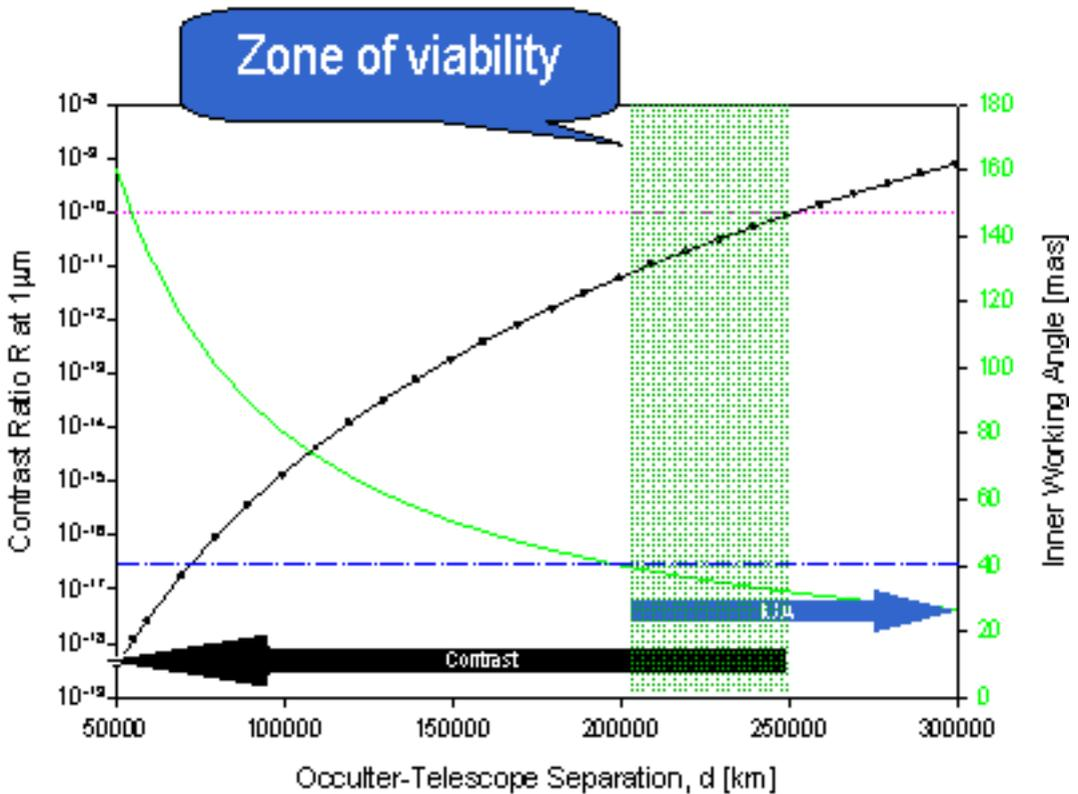
Figure 4. Contrast Ratio and Inner Working Angle versus Occulter to Telescope Separation.
