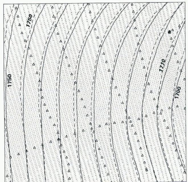
Fig. 2. ALTM elevations (dots) and derived elevation contours (solid lines) within a 500 m  $\times$  500 m area A1, together with ground-based GPS elevations (triangles) and derived elevation contours (dashed lines). North is upwards. Contour interval is 5 m, with elevations in m a.e. (above WGS84 ellipsoid).
