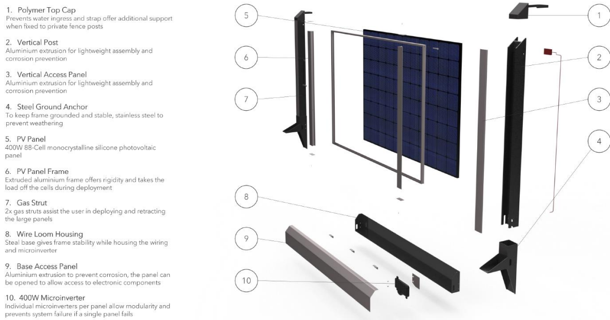
Figure 6. Edge Solar technical solution per panel
