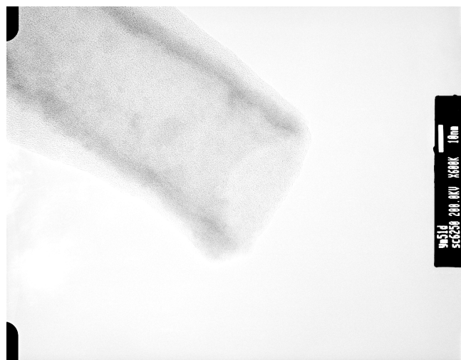
Figure 3. High resolution transmission electron microscope (HRTEM) image of an empty bismuth-oxide shell, remaining after the HCl acid dip.
