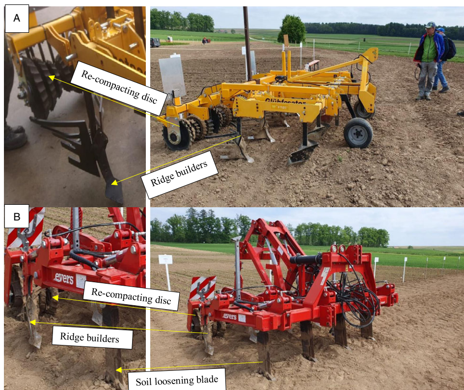
Figure 2. Real-time kinematic global navigation satellite system (RTK-GNSS) ridgers used in the experiments. A) Glühfosator, an RTK-GNSS guided ridger for creating and re-compacting ridges (Frost Maschinenbau GmbH, Petershagen, Germany). B) DammProfi, an RTK-GNSS guided ridger for seeding, soil loosening (up to 0.5 m depth) and creating re-compacted ridges (Evers GmbH, Oberhausen, Germany).
