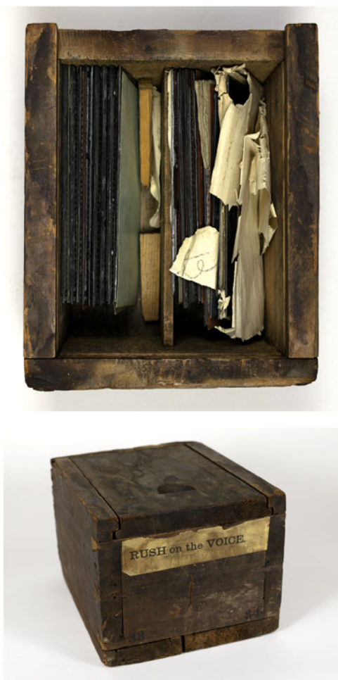
Figure 3. Interior and exterior views of a typical box for the storage of stereotype plates. Here 22 plates are organized into 11 pairs: the smooth sides are placed back-to-back, with the text sides facing outwards. This box stores some of the plates for James Rush, The Philosophy of the Human Voice (Philadelphia: J.B. Lippincott & Co. [with the cooperation of the Library Company of Philadelphia], 1855. 10 x 8 x 6.5 inches. Library Company of Philadelphia.
