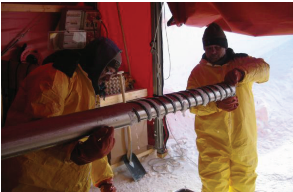
Fig. 20. Core barrel being extracted.
