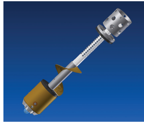
Fig. 4. Hollow shaft within chip chamber with spiral booster.
