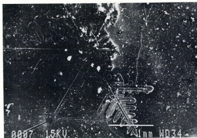
Fig. 2. SEM image of a captured snow crystal.
