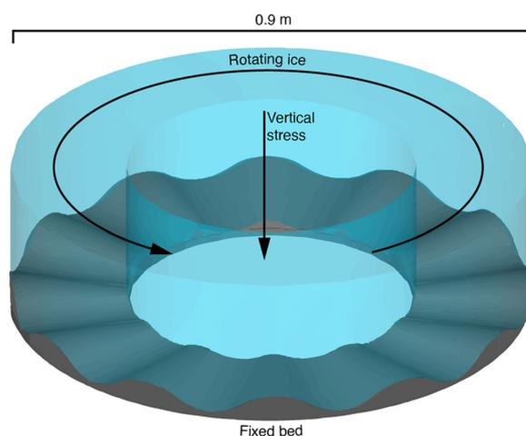
**Fig. 2.** Schematic of the bed and ice ring used in these experiments. A ring of ice, 0.9 m in outer diameter, is pressed against a sinusoidal bed made of Delrin. The ice ring is gripped at its upper surface by a platen and dragged over the bed, which is fixed rotationally but moves up or down as the volume of the ice chamber that holds the ice ring changes due to changes in cavity size. The bed is designed so that adverse slopes of bumps do not vary radially.
