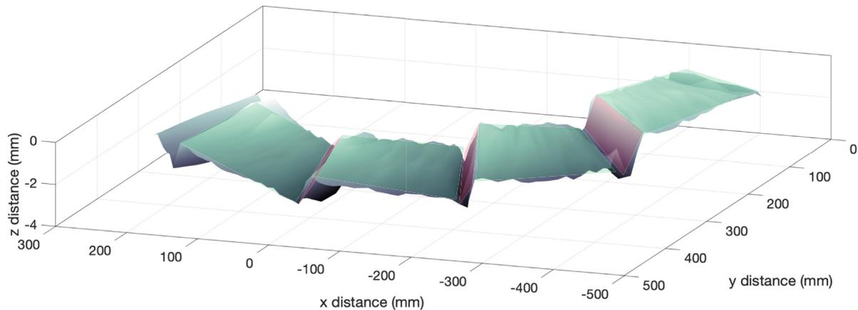
**Fig. 4.** Cavity geometry. Morphology of a portion ( $\sim 1/4$ ) of the ice sole measured at the final sliding speed ( $290 \text{ m a}^{-1}$ ). In this plot, the shaded green sections represent the cavity roofs, and the shaded pink sections represent the areas where the ice was in contact with the uppermost, up-glacier-facing parts of bumps on the bed like those shown in Figure 2.
