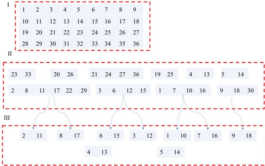
Figure 26. Feature selection procedure illustration using rough surface indices. Each number here is representative of a rough surface: I denotes the initial stage involving all surfaces in the group; II denotes the next stage after one feature RI_x/k_a was selected; and III denotes the third stage when ES is selected.
