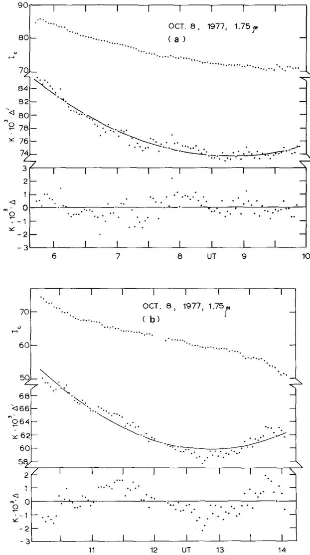
Fig. 6a–b. The plot of originally recorded calibration signal  $I'_c$  (top), of the ratio  $K\Delta' = \delta'/I'_c$  together with the least squares fit by parabola (middle) and of the residuals  $k\Delta$  (bottom), vs UT.
