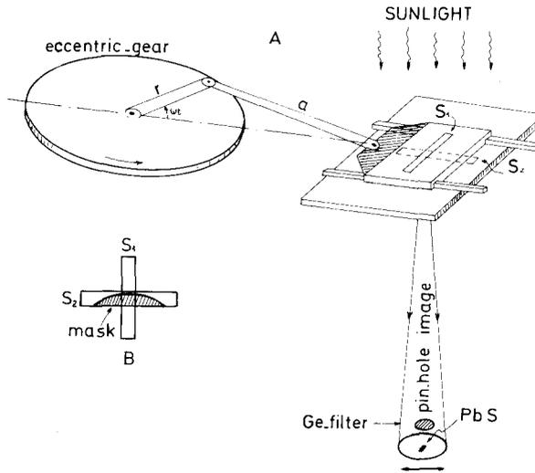
Fig. 2. Schematic drawing of the device used for the IR intensity measurements (dimensions are quite arbitrary); for the explanation see text.
