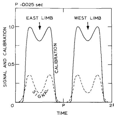
Fig. 4. Modulation pattern of the PbS output with the use of a profiled mask (see text).
