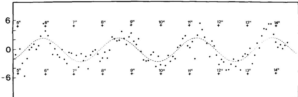
Fig. 7. The averaged measurements of 1977 (a total of 156 hr corresponding to 32 days) arranged using the superposed epoch method. Time is UT and amplitude is in units of  $10^{-4}$  of the 'average Sun'. Dotted line represents the best fitted 160-min sinusoid.
