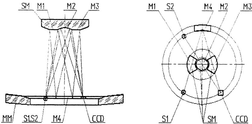
Fig. 1. Optical scheme of the Secondary Alignment System.
