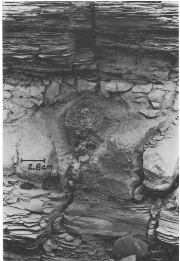
Figure 5. Coarse analcime nodule that replaced the surrounding alkalic zeolites in the tuff (ZT). Note the fractures in the underlying oil shale. These fractures served as pathways for concentrated brines emanating from the underlying evaporite facies (Buff Marker Bed of Figure 3).
