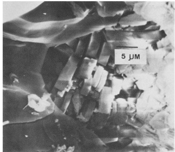
Figure 11. Scanning electron micrograph showing heulandite laths (edge view) adjacent to a glass shard.
