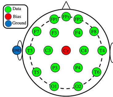
Figure 3. Electrode locations used to capture EEG data, locations based on the 10-20 system of measurement
