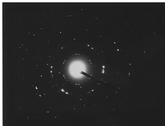
Figure 5. SAED pattern of CHT sample calcined at 773 K and left in contact with 0.1 M NaI- ^{131}\text{I} , 733CHT-I solution.
