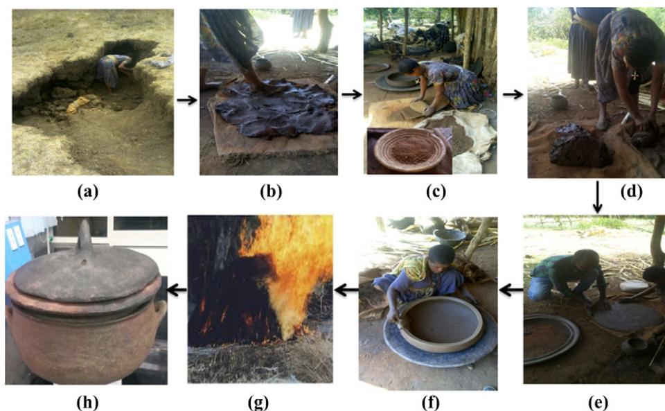
**Figure 2.** Photo image of the procedure for preparing and shaping a mosseb-designed Zeer pot: (a) Digging clay, (b) Making fresh clay mud, (c) Grounding old clay, (d) Mixing clay with old clay powder to make a better mud, (e) Designing a mosseb-like Zeer pot, (f) Drying a mosseb-designed Zeer pot, (g) Mosseb-designed Zeer pot firing and (h) Finished a mosseb-designed Zeer pot.
