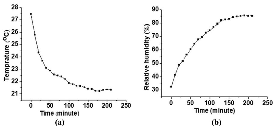
**Figure 4.** Temperature versus time (a) and humidity versus time (b) graph of the designed evaporative cooler.
