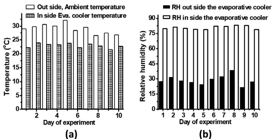
**Figure 5.** Average temperature (a) and relative humidity (b) versus the day of the experiment of the cooler and the ambient.
