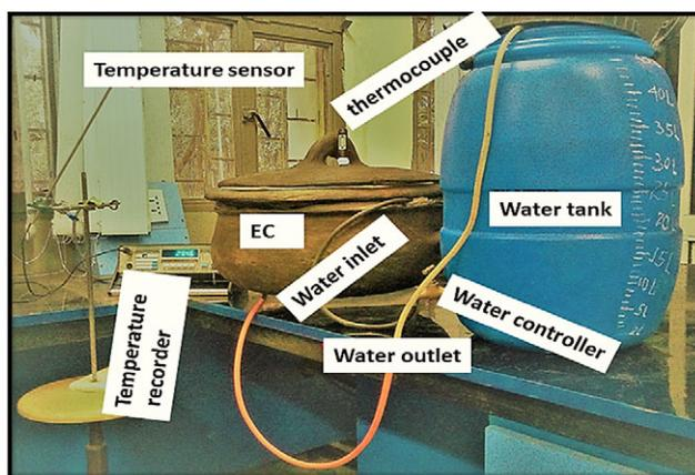
**Figure 3.** Complete setup of the mosseb-designed evaporative cooling chamber.
