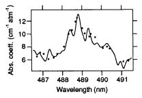
Figure 2. Comparison of our measured  $NO_2$  absorption coefficient (solid line) and that published by Woods and Jolliffe (1978) (points).
