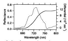
Figure 1. The red edge of a green-plant reflectance spectrum (solid line, left axis) and its first derivative (dotted line, right axis).
