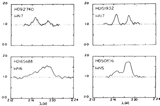
Fig. 3 CGS spectra showing BY and HeII(14-8) at  $2.165\mu$  and HeII(10-7) at  $2.189\mu$ .
