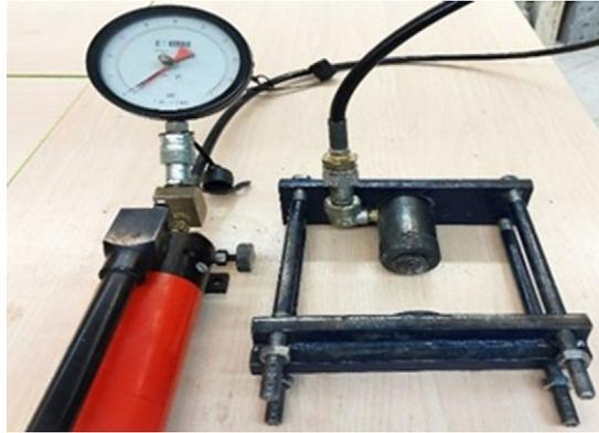
**Figure 3.** Hydraulic jack and metal frame for confining pressure applications.
