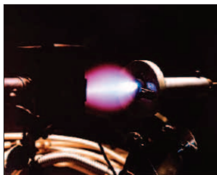
Figure 1. Typical plume emitted from the interaction of a laser with a YBCO target material in the pulsed laser deposition process.
