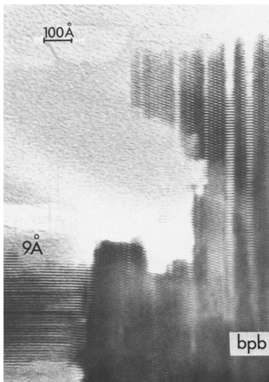
Figure 3. Layer silicate (9-Å) in crystallographic continuity with a complex series of biopyriboles.
