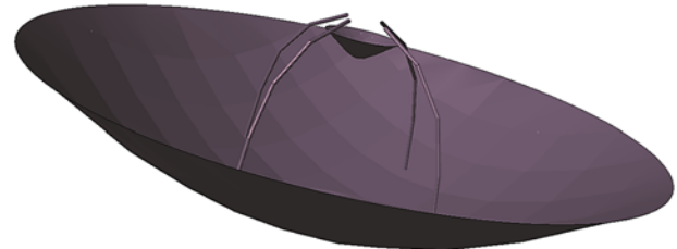
Figure 9. DSA4 GRASP model of main- and sub-reflector, with the inner part of struts.
