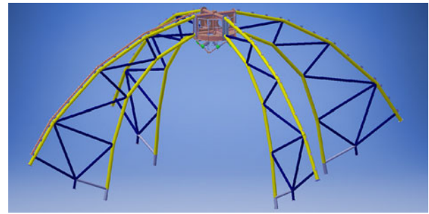
Figure 8. DSA4 struts, CAD model.
