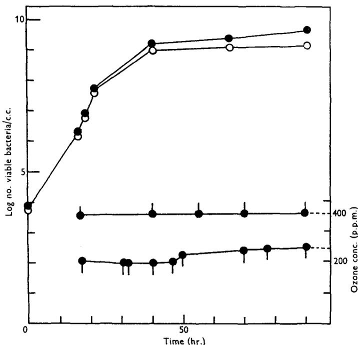
Fig. 5. The continuous consumption of ozone at 20° C., by an active culture of *Achromobacter* (a rate of the order of  $10^{-11}$  g. ozone/hr./cell is suggested). ○, air control; ●, air + ozone 380 p.p.m.; ●, ozone entering flask; ●, ozone leaving flask.
