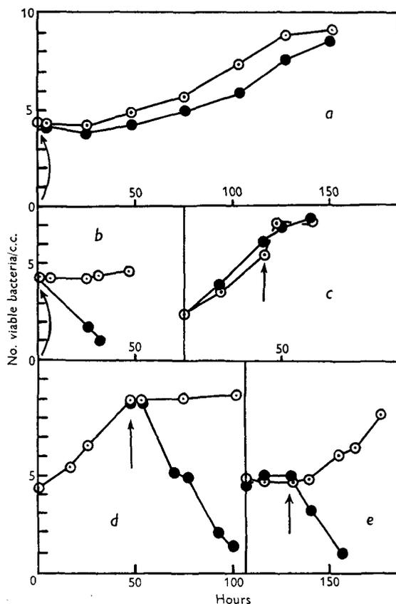
Fig. 3. The effect of ozone on *E. coli* in Nelson's medium at 20° C. (a) 4 p.p.m.; (b) 10 p.p.m.; (c) 190 p.p.m.; (d) 680 p.p.m.; (e) 715 p.p.m. by volume. The time at which the ozone was first admitted is indicated by the arrows. ○, air control; ●, test with ozone.
