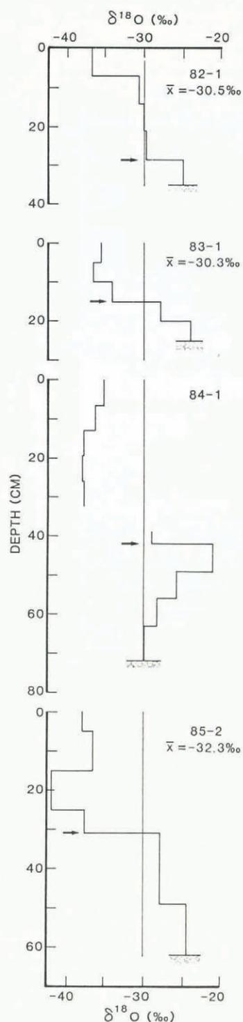
Fig. 3.  $\delta^{18}\text{O}$  profiles of snow pits at one location at the west end of Ward Hunt Ice Shelf, 1982–85 (see Fig. 1). Arrows mark the top of the depth-hoar layer.
