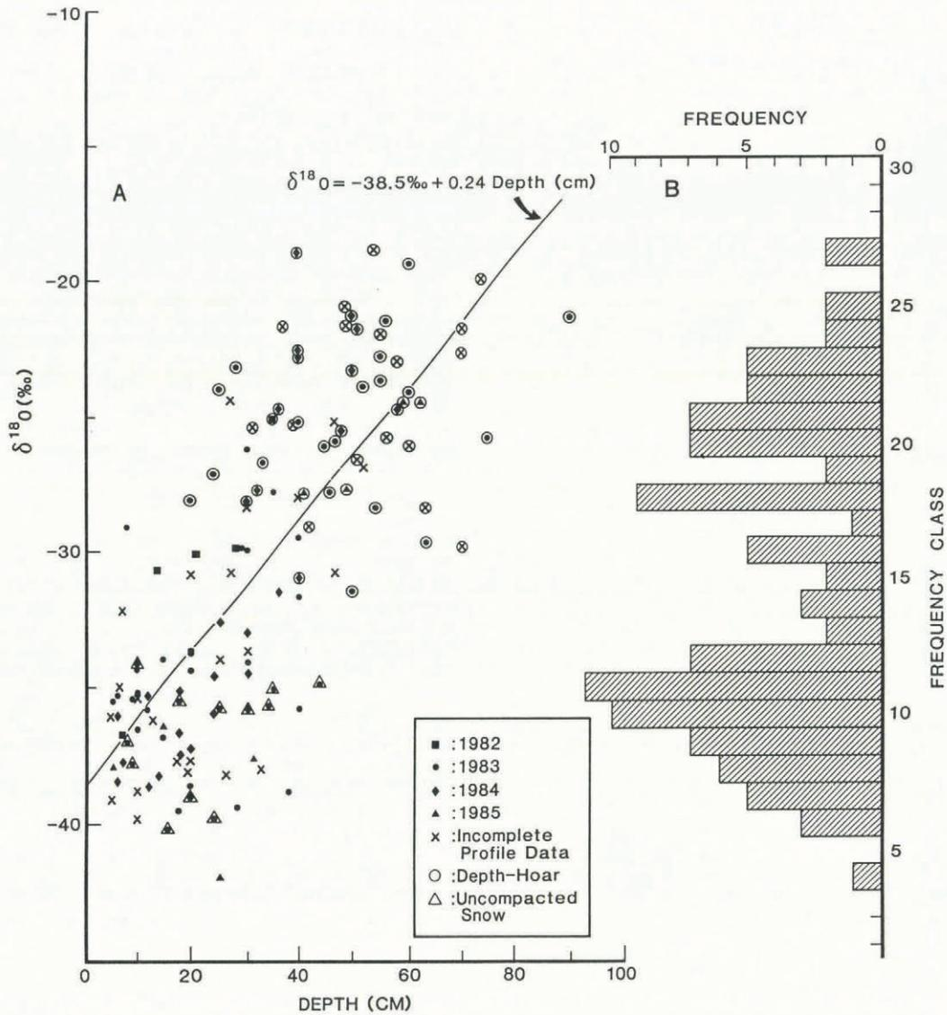
Fig. 4. a. Relationship between snow  $\delta^{18}\text{O}$  values and depth at which samples were obtained. b. Frequency distribution of  $\delta^{18}\text{O}$  values. The frequency classes are at  $0.99\text{‰}$  intervals, e.g. class 10 represents  $-35.49\text{‰}$  to  $-34.5\text{‰}$ , class 15 represents  $-31.49\text{‰}$  to  $-30.5\text{‰}$ , and class 20 represents  $-26.49\text{‰}$  to  $-25.5\text{‰}$ .
