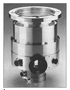
Maintenance-Free Turbomolecular Pump: The Turbovac® 1000MC from Leybold Vacuum Products is designed for research, instrumentation, particle beam accelerator, plasma etch, and coating applications. A permanent magnetic passive bearing suspends the pump rotor, and the pump shaft position is monitored by an axial sensor which continuously adjusts the rotor position in the event of deviation. The device features convection cooling and two lubricant-free bearings which stabilize the rotor shaft.
