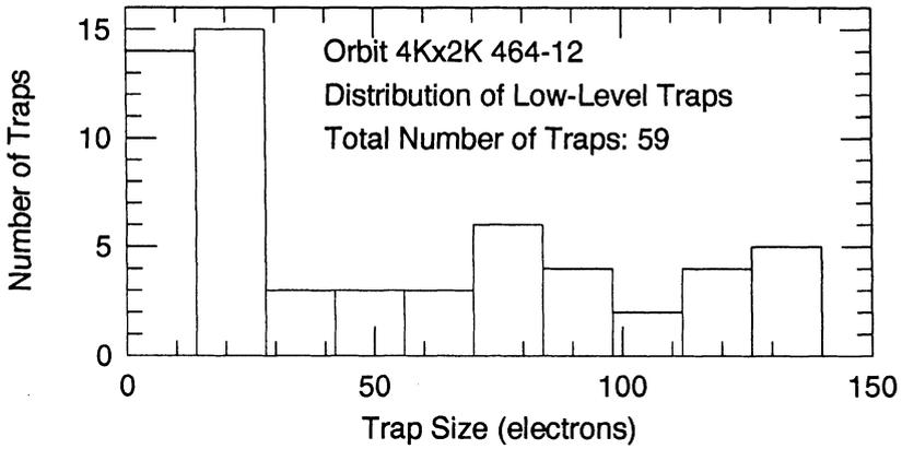
Fig. 2. Size Distribution of Localized Traps
