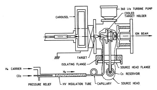
Fig. 1. Schematic layout of the CO<sub>2</sub> ion source
