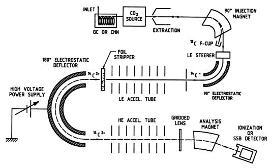
Fig. 4. Schematic layout of the HVEE <sup>14</sup>C AMS spectrometer
