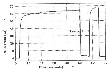
Fig. 3. Analyzed <sup>12</sup>C<sup>-</sup> ion source current as a function of time for two different graphite samples
