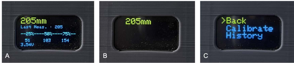
FIGURE 3. LCD screen on PODv1 including (A) Live Measurement display screen, (B) Precision Mode, and (C) Calibrate and History.
