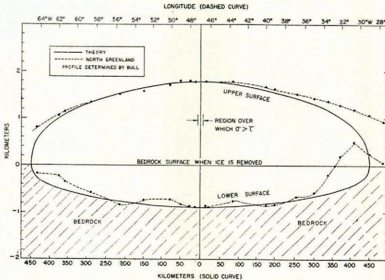
Fig. 1. Profile of a large ice sheet. Solid curve: Theoretical profile of a large ice sheet for which the bedrock is in isostatic equilibrium. If the ice were removed, the bedrock surface would be flat. Dashed curve: Profile of the north Greenland Ice Sheet at about lat.  $78^\circ$  N. as determined by Bull.<sup>11</sup> (Elevation scale has an arbitrary origin. Altitude above sea-level of the center of the ice sheet is 2,527 m. at the top surface and  $-153$  m. at the bottom surface)
