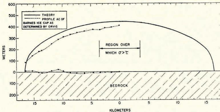
Fig. 2. Profile of a small ice cap. Solid curve: Theoretical profile of a small ice cap with a flat bedrock surface. Dashed curve: Profile of one section of the Barnes Ice Cap as determined by Orvig.<sup>12</sup> (Elevation scale has an arbitrary origin. Altitude above sea-level at position 0 km. is 866 m. for the surface and 409 m. for the lower surface)
