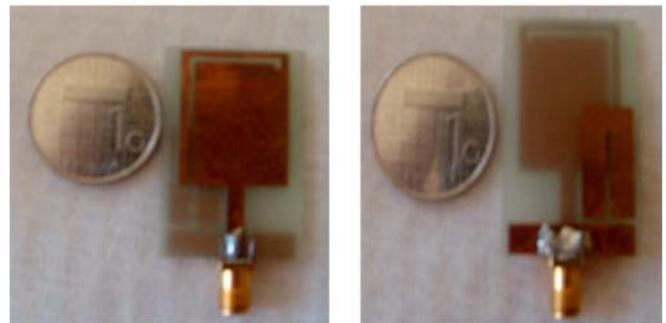
Fig. 6. (Color online) Geometry of the proposed final antenna.
