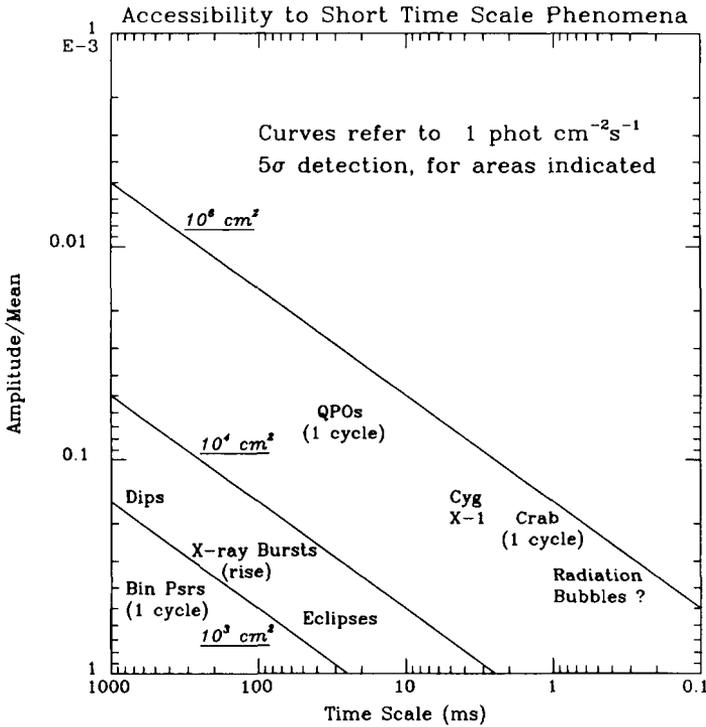
Fig. 1. Low amplitude and short timescale variability require large area instruments, such as XLA, to be detected. Currently planned X-ray timing missions are all smaller than  $10^4 \text{ cm}^2$  in area; XLA has an area of  $10^6 \text{ cm}^2$ .
