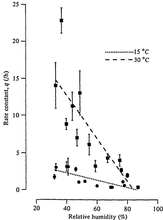
Fig. 2. Rate constants for second-stage death of aerosolized *Escherichia coli* vs relative humidity. Bars denote 1 s.e.
