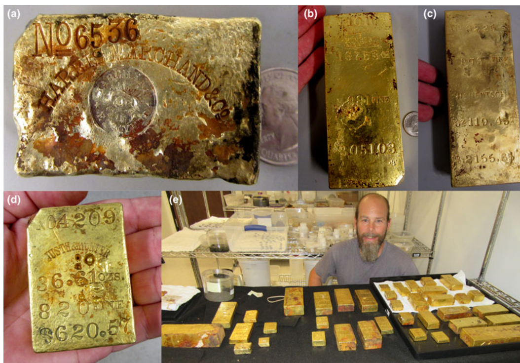
Fig. 3. Images showing the variety of gold assayer's ingots from different assay houses (Table 1) included in this study: (a) Harris, Marchand & Co. Ingot #6536, prominently displaying the French assayers' stamp. The missing upper left corner is material removed in 1857 to generate the stamped assay value on the side edge (hidden in view). Reddish-black patches are iron coatings from the shipwreck. Coin is 24.3 mm. (b) Kellogg & Humbert Ingot #1010 with hand and 24.3 mm coin for scale. Assay chip is from lower right corner. This ingot, and the following two, show the typical format of period assayers' ingots, with stampings on the front which denote assay house, ingot number, fineness expressed as three digits, mass in troy ounces and dollar value based on period value of USD$20.67 per troy ounce. (c) Assay Office of Henry Hentsch Ingot #3225 with hand for scale. Assay chip is from upper right corner. (d) Justh & Hunter Ingot #4209, with hand for scale. Assay chip is from the upper left corner. (e) Over 75 kg of gold in 37 assayer's ingots from the the SS Central America with lead author for scale. Photos by the authors, and with permission of California Gold Marketing Group.
