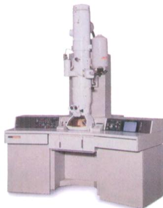
JEM-2010 Transmission Electron Microscope
