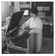
**ON THE COVER**: Laser Raman microprobe system (Jobin-Yvon/Atago Bussan) used at the Tokyo Institute of Technology for analyzing corroded and coated surfaces of advanced materials. The technician is adjusting the optical system. Spectra of a 70-nm-thick carbon layer formed under hydrothermal conditions on SiC fibers are shown. For more information about this topic, see "Water Effects on Corrosion Behavior of Structural Ceramics" by Y. Gogotsi and M. Yoshimura on p. 39.
