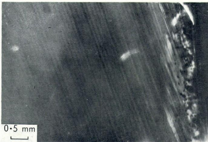
Fig. 3. Interference bands parallel to slip lines.
