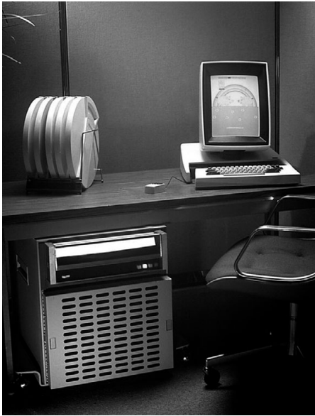
Figure 3.9 Alto with storage disks, computer, vertical display, mouse and a keyboard. (Source: Computer History Museum. Courtesy of PARC. Reproduced with permission of SRI International)
