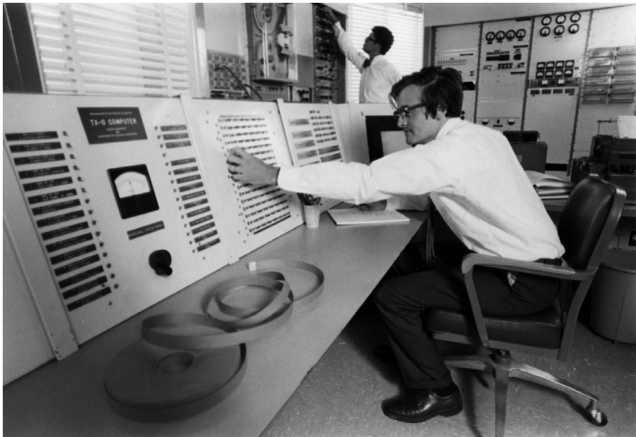
Figure 3.4 TX-0 with the control panel, including the Toggle Switch Storage, 12 1/2" cathode-ray oscilloscope display tube and Flexowriter teletype terminal behind the operator. (Source: Courtesy of the Computer History Museum)
