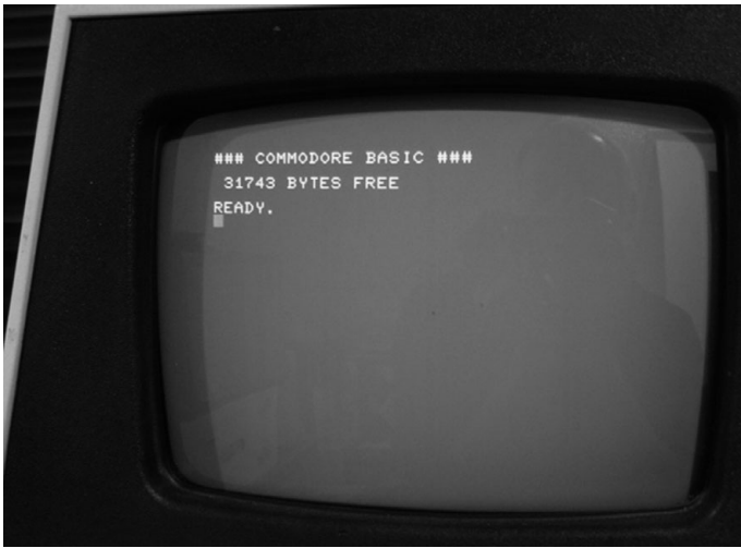
Figure 3.14 After turning on, Commodore PET starts and immediately runs Commodore BASIC. Any further interactions were through the BASIC command prompt. (Source: Courtesy of Terry Stewart. 103 Reproduced with permission)
