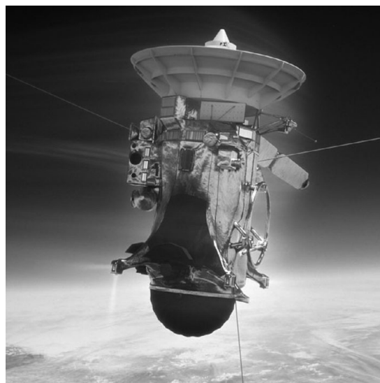
Figure 1.11 The nuclear-powered Cassini spacecraft, launched towards Saturn in 1997, was active for nearly 20 years. The ring on the right side held the Huygens probe, which parachuted onto Titan's surface. NASA image. For the colour version, refer to the plate section.
