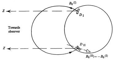
Fig. 3. Measurement of the Zeeman effect in two regions,  $D_{I}$  and  $D_{II}$ , of the sun equally distant from the equatorial plane and situated on the same meridian circle. The observer is situated approximately in the equatorial plane. The general magnetic field  $B_0$  is assumed to have a dipole-like shape.
