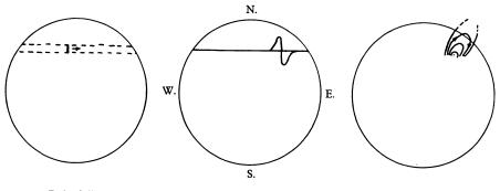
Path of slit Deflexion on a BM region Inferred flux loops Fig. 1. Response trace of magnetograph as slit scans image.
