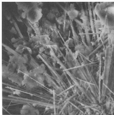
Figure 9. Acicular crystals of xonotlite formed on the surface of a thick pellet (~3 mm) of hisingerite material after treatment at 370°C and 13.8 MPa water vapor pressure for one week.
