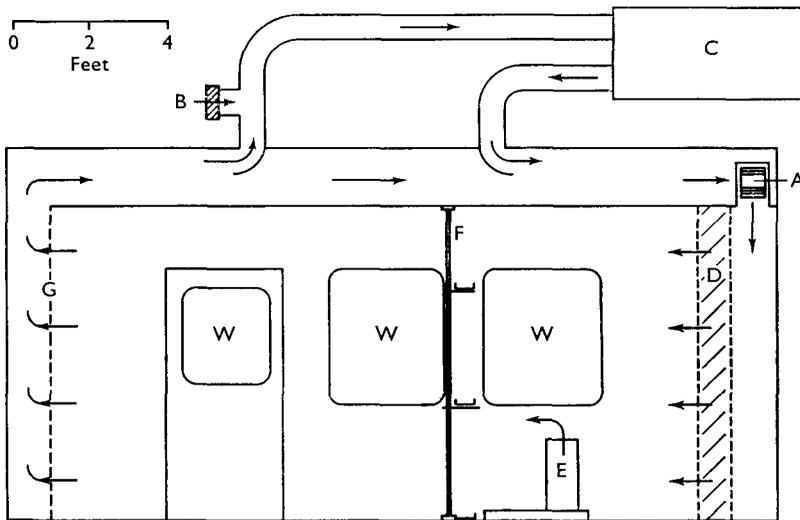
Fig. 1. Section of room. A, Recirculating fan; B, make-up air inlet; C, air-conditioning unit (temperature and humidity control, including a refrigeration unit); D, filter bank (prefilter followed by high efficiency filter); E, airborne particle generator; F, stand with sampling plates; G, return grille.
