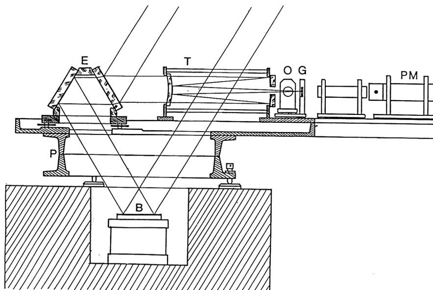
**FIGURE 1.** The photoelectric astrolabe: B= Mercury bath, P= Bearing, E= Angle standard, T= Maksutov-Cassegrain Reflector, O= Monitoring eye piece, G= Modulation Grid, PM= Photomultiplier.
