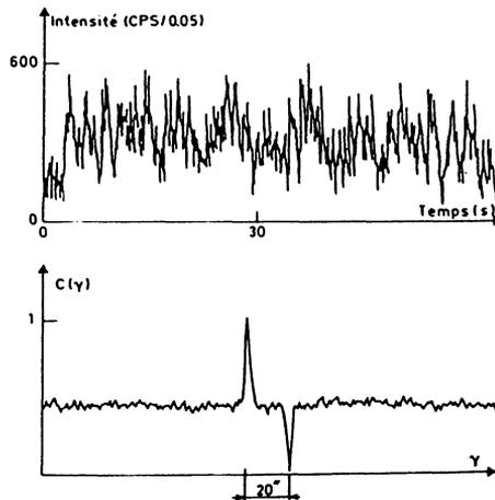
FIGURE 5 - The pseudo-noise grid. The grid consists of 60 slits, built with 262 elementary steps of 25  $\mu\text{m}$ . The upper part shows the signal intensity as a function of time. In the lower part the autocorrelation signal between the reference grid and the record is shown.
