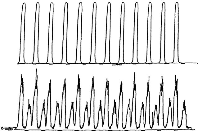
**FIGURE 2** - Transit of a star. The upper part shows the transmission of a 12 slits grid while the lower part shows the actual record for both images with the same grid.
