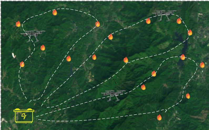
Figure 1. Persistent monitoring scenario, where multiple UAVs are used to monitor wildfire situations and return to a fixed base station for replacing the battery at the end of their energy cycle.
