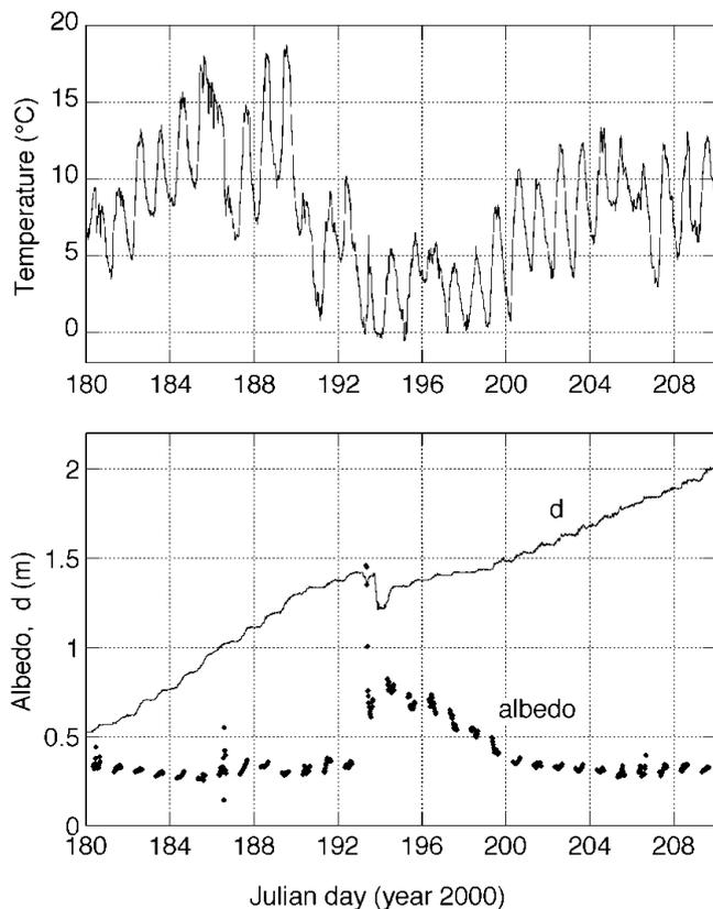
Fig. 2. Meteorological records from the AWS on the snout of Morteratschgletscher (site 1). The upper panel shows air temperature at  $\sim 3.5$  m above the glacier surface. The lower panel shows the distance to the surface ( $d$ ) measured with the sonic ranger and the surface albedo (half-hourly values only for 0800–1600 UT).
