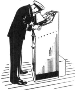
The s.s. 'Maturata', like so many ships today, relies on BTH Radar for safer all-weather navigation. She is equipped with Type RMS2 and a 12-in. display. For passage up the Manchester Ship Canal the mast and scanner unit can be lifted out and stowed.
