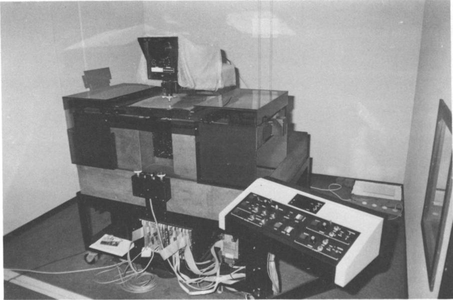
Fig. 1. The 2020GM PDS microdensitometer at Muenster
