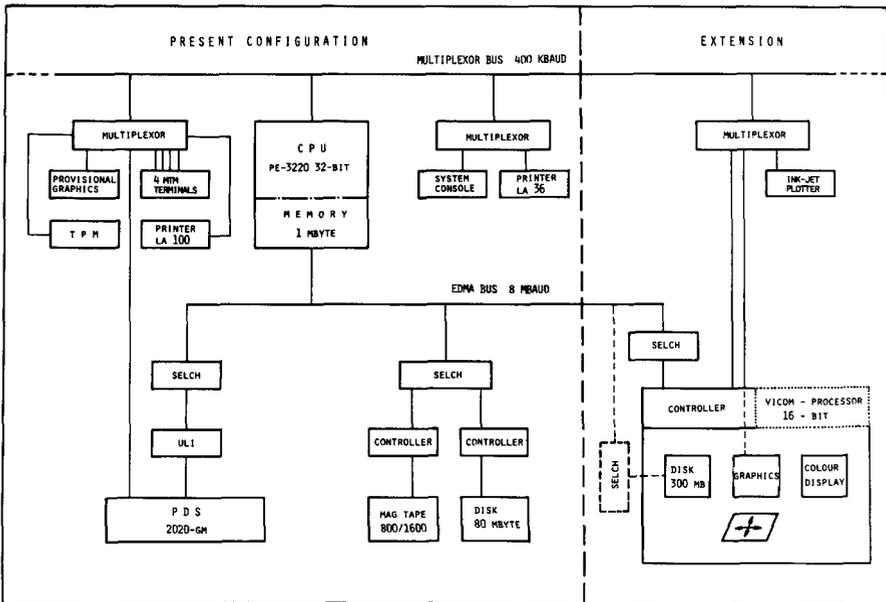
Fig. 2. The system configuration including the 2020GM PDS
