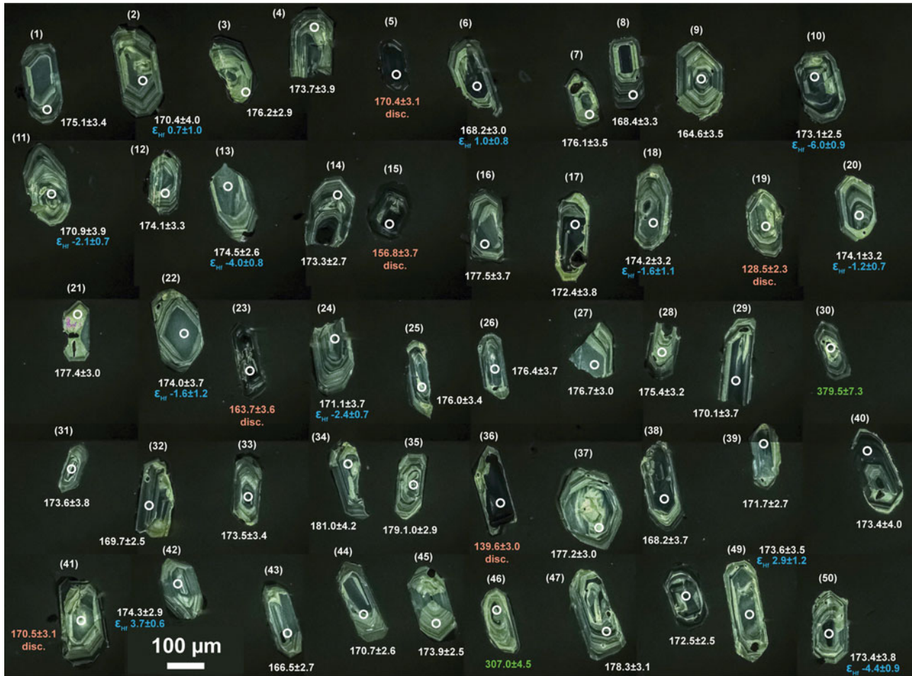
Figure 5. Cathodoluminescence images and U-Pb dates of the 50 zircon grains analysed from sample SIA (SI = Sif Island). Red text indicates discordant ages, and the two Palaeozoic inherited cores are highlighted using green text. Also shown are the \epsilon_{\text{Hf}} values (blue text).
