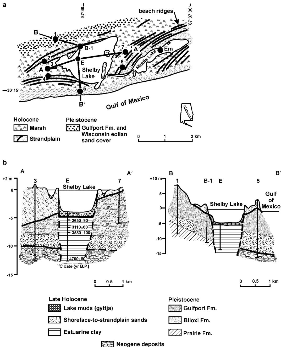
FIG. 2. (a) Shelby Lake, southeastern Alabama. Geologic units and drillhole locations are from Otvos (1999). (b) Geologic cross sections across Shelby Lake. Core E, with radiocarbon dates and general geology during Hurricane Opal are reproduced from Liu and Fearn (1993) and Otvos (1999).
