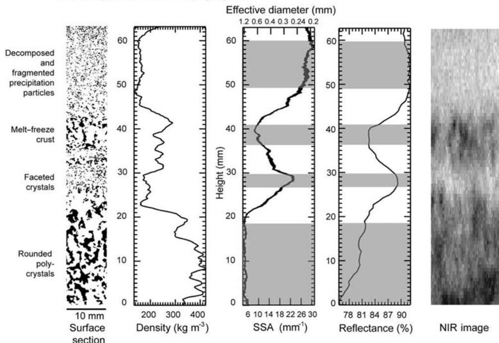
**Fig. 2.** Surface section and NIR image of two snow samples and the derived density, specific surface area (SSA) and reflectance signals. For sample 2 the absolute height of the surface section and the NIR image vary. The grey bands mark visually identified layers.
