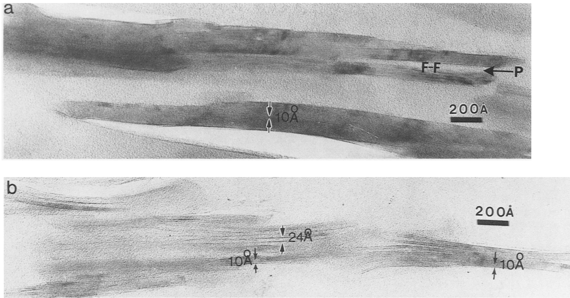
Figure 14. Lattice-fringe images of an illite (IMt-1): a) Na-treated and b) dodecylammonium ion exchanged. In (b), many 10 Å layers have been expanded to 24 Å. Pores (P) associated with layer organization (F-F = face to face) are shown.
